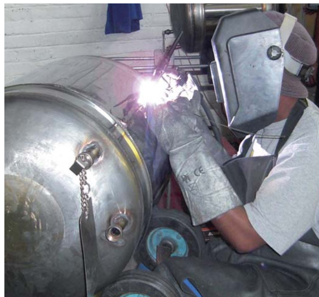
Welding a Type 430 heat exchanger onto a Type 444 inner tank
